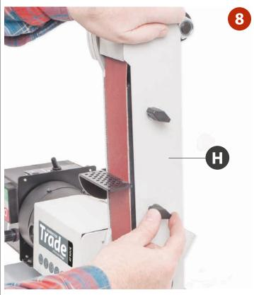
Replace the belt 'Access Plate' (H) and secure in place with the two butterfly threaded knobs
