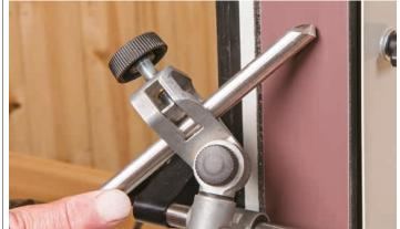
Many of the Tormek<sup>®</sup> jigs work amazingly well on the 12mm bar of the Ultimate Edge and provide the user with extremely sharp and accurately ground tools. The Tormek fingernail grinding jig is shown using an aluminium oxide belt with a 65mm protrusion. See the Tormek<sup>®</sup> pages for full details.
