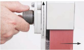
Turning the tracking knob anti-clockwise moves the belt to the right
