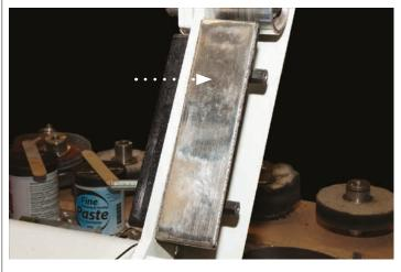
**5.** Slide the belt back on the drive rollers and centre the belt on the linisher. Press the lever (2) down and hold in place, pull the locking 'PIN' (3) out and raise the linisher's head to re-tension the belt, see fig 17.
