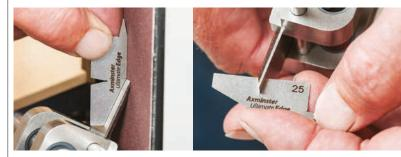
As with all accurate sharpening, it's all about the angles and our 18 piece set gives all angles from 90° through to 5°. The set is perfect for setting up sharpening guides as well as checking ground angles. The UJK level box is an additional useful accessory for the Ultimate Edge, its ability to record and set angles is perfect for this application.
