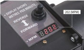
**4.** Turn the speed control knob until the display reads around '400' (MPM), see fig 23
