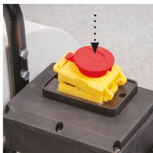
Emergency Stop Press down to stop the machine
