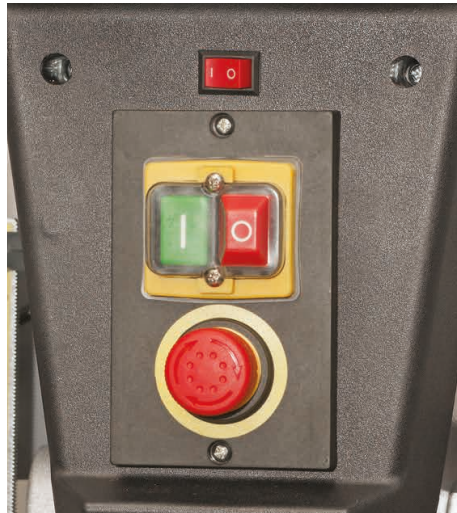
ATDP20F pillar drill control panel NOTE: The LED light switch is above the On/Off switch assembly
