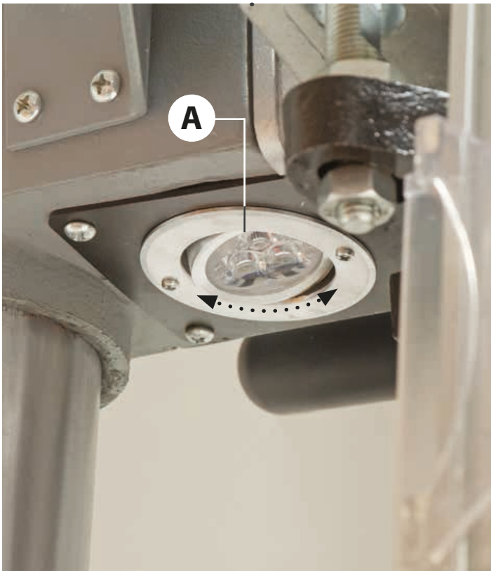
LED light (A) below the drill head pivots to direct light down onto the work table
