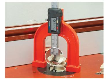
Setting the router cutter height in the router table, see top picture.
