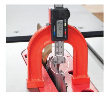
· Setting the blade height on the panel saw, see picture above.
