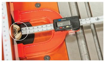
• Setting the distance of the bandsaw fence from the blade, see picture below.
