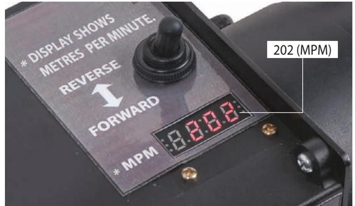
4. Turn the speed control knob until the display reads around '400' (MPM), see fig 23
