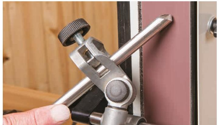
Many of the Tormek® jigs work amazingly well on the 12mm bar of the Ultimate Edge and provide the user with extremely sharp and accurately ground tools. The Tormek fingernail grinding jig is shown using an aluminium oxide belt with a 65mm protrusion. See the Tormek® pages for full details.
