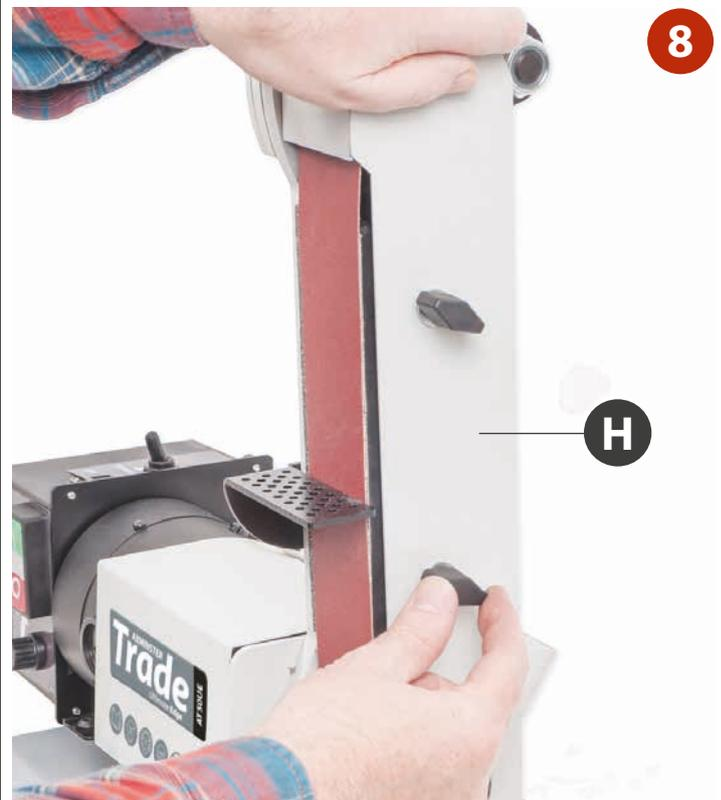
Replace the belt 'Access Plate' (H) and secure in place with the two butterfly threaded knobs
