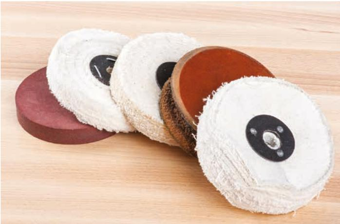
A variety of 12mm bore accessories are available for use on the "Twist n Fix" 12mm arbor including a leather profiled wheel for carving tools, a rubberised wheel for polishing and traditional mops both stitched, loose leaf and sisal. N.B. Smaller sizes of abrasive soaps are available online.
