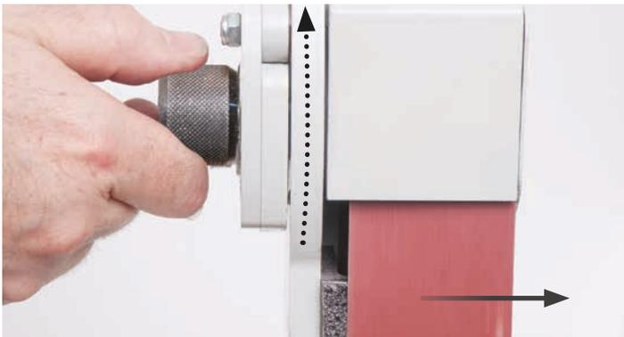
Turning the tracking knob anti-clockwise moves the belt to the right
