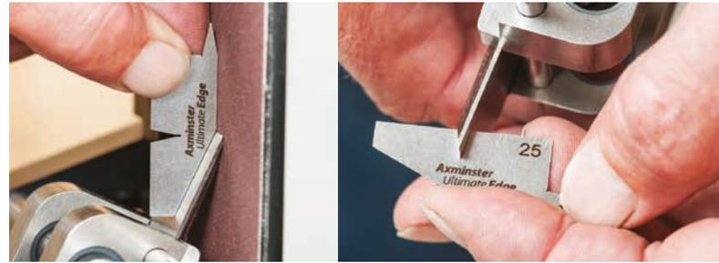
As with all accurate sharpening, it's all about the angles and our 18 piece set gives all angles from 90° through to 5°. The set is perfect for setting up sharpening guides as well as checking ground angles. The UJK level box is an additional useful accessory for the Ultimate Edge, its ability to record and set angles is perfect for this application.
