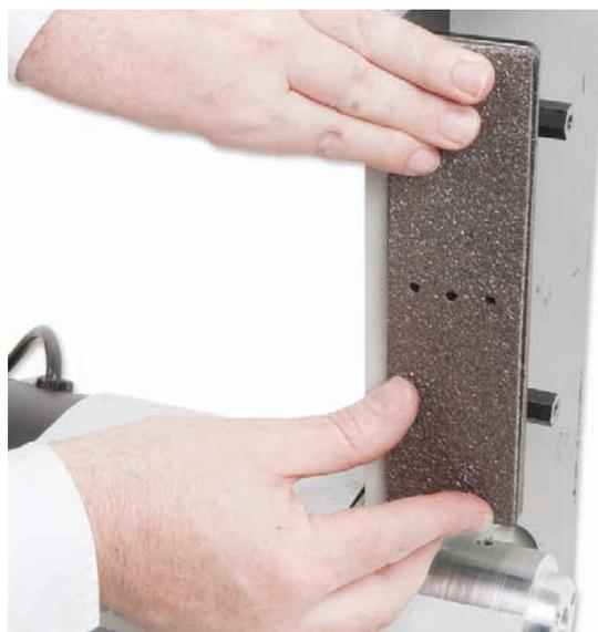
**Note:** After a period of time the 'Graphite Pad' will become worn and we recommend fitting the optional 'Slip Plate', code 105676, see picture below.
