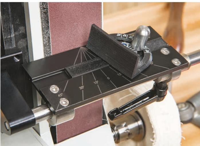
This table is an accessory for the Ultimate Edge Compound Jig. This is machined from anodised alloy and is supplied with a mitre setting guide. The table is locked by a handle locking securely onto the round bar. Anodised in black, there is a quadrant of angles laser marked into the surface for easy reference. Ideal for freehand lathe tool sharpening and general finishing. Size 130 x 75mm.
