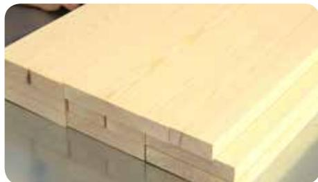
The first step in creating your own neon resin plank table is to choose the wooden planks you wish to use - this will depend on the size of the piece you wish to create and the look you wish to achieve. You may need to cut down some of the planks to give a balanced mix of long and short planks, or a mixture of widths.
