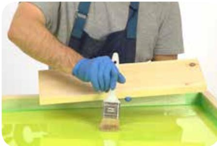
As you lower the planks tilt them on the long edge and lower slowly with a slight rocking motion until the plank is sitting on the resin. This will help to prevent air pockets being trapped on the underside of the planks.
